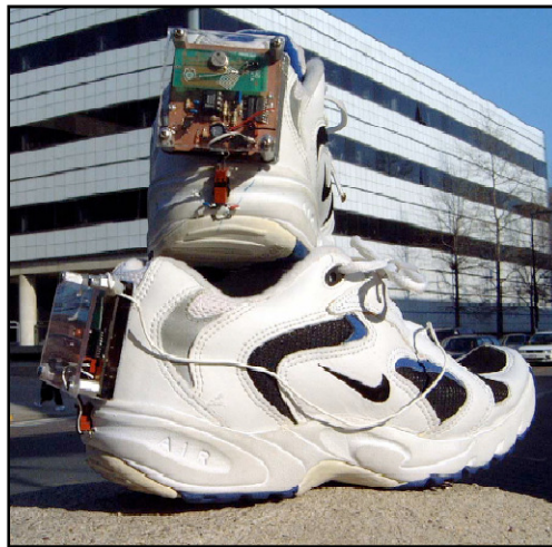
Figure 6. Power Generation Using a Piezoelectric Source in a Shoe [7]
