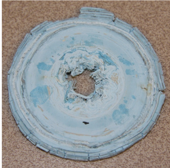
Figure A6. First Coil Prototype Compressed by the Uni-Axial Press
